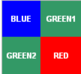
Figure 3. Color Filter Arrangement on the Pixels
